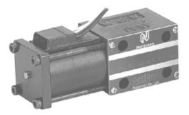
**Description** 4 Way - 3 Position- Spring Centered Mobile Transmission Hydraulic Valve, Float Center Spool, ISO 03/NFPA D03/NG6 Mtg Pattern, Push-Pull Coil Series, Push Rod Solenoid End.
