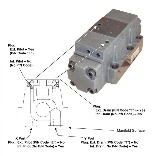
At conversion, the one plug that is removed may be used as the other required plug.
